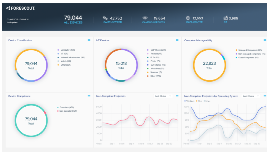
Figure 5: The Forescout platform's customizable web dashboard provides IT and security operations teams with a comprehensive view of devices, their classification context and their security posture, allowing for real-time risk prioritization.
